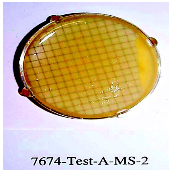
Figure 9. MS-2 Phage Culture Exposed in Test Unit for Approximately 24 hr
